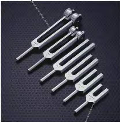
Tines with small mass m : high frequency f = 4096 Hz
